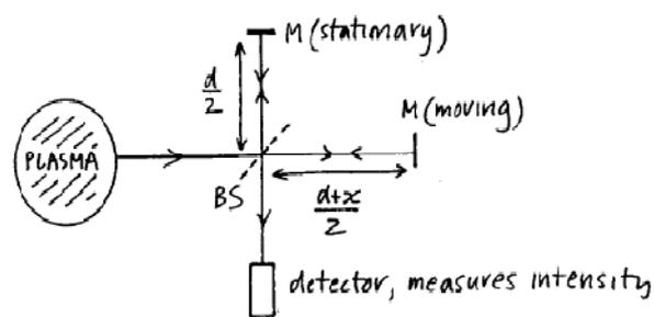
Figure 5: Scheme for measuring the intensity of wave emission from plasma fusion (Michelson interferometer systems).
