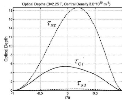
Figure 3: The optical depth  $\tau$  for O1, X2, X3 modes [10].
